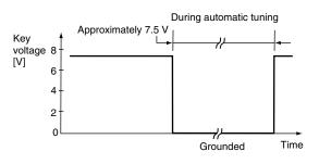
If the key voltage is more than 8 V, switch the [MODE] switch (J31) to OFF mode\*.
