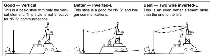
\*Near Vertical Incidence Skywave. This is a radio-wave propagation method that provides usable signals in the range between groundwave and skywave distances (usually 30 to 400 miles, or 50 to 650 km).
