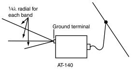
$^{1\!/\!4\lambda}$  (quarter wavelength) radial for each band is suitable for a counterpoise. Install the counterpoise directly below the AT-140's ground terminal. Insulate the ends of each radial from other metal objects. Layout the radial horizontally and as straight as possible.
